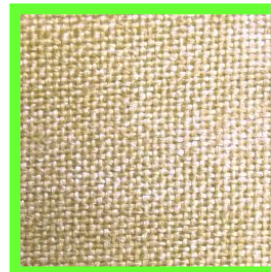
1500F / 815C Fiberglass with Vermiculite Fabric. Page 4-13
