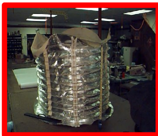
Lift Cylinder Bellows Protection Page 7-5
